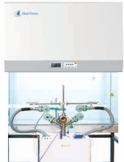
KI-discus containment test 2
